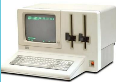
The Datamaster was an all-in-one computer with text-mode CRT display, keyboard, processor, memory, and two 8-inch floppy disk drives all contained in one cabinet. (Photo: Oldcomputers.net)
