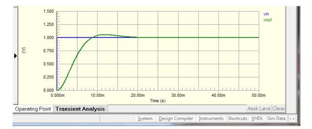
13. We can also make measurements on these waveforms. Click the name "vout" on the right side of the plot (red arrow). This selects just that signal or "wave." Go to Wave → Cursor A and Cursor B to turn on both cursors. You should now see measurements in the Sim Data panel, as well as on the bottom of the chart (purple arrow).
