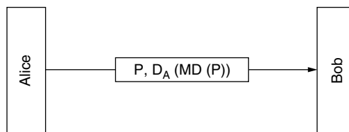
Figure 8-20. Digital signatures using message digests.
