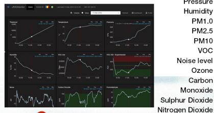
Temperature Pressure Humidity PM1.0 PM2.5 PM10 VOC Noise level Ozone Carbon Monoxide
