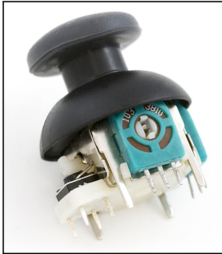
Figure 3-2: a simple joystick sensor
