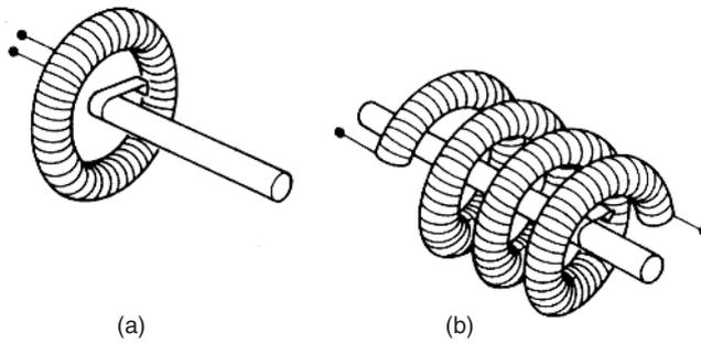
Fig. 20.1 Rotary motion potentiometers: (a) circular; (b) helical.
