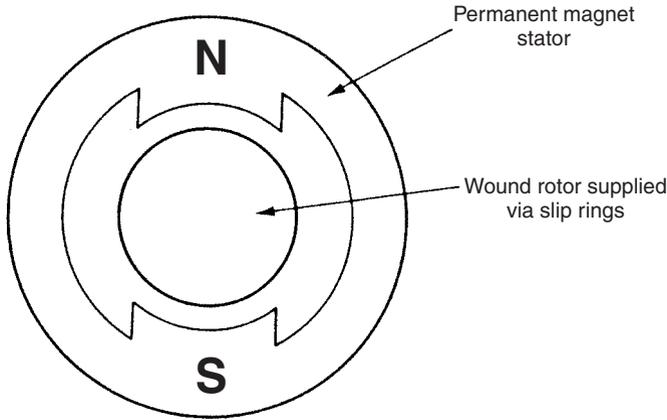
Fig. 20.19 D.c. tachometer.
