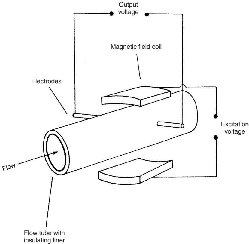
**Fig. 16.10** Electromagnetic flowmeter.
