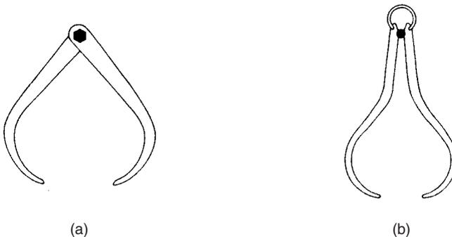
**Fig. 21.3** (a) Standard calliper; (b) spring-loaded calliper.
