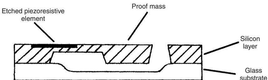
Fig. 13.15 Silicon microaccelerometer.
