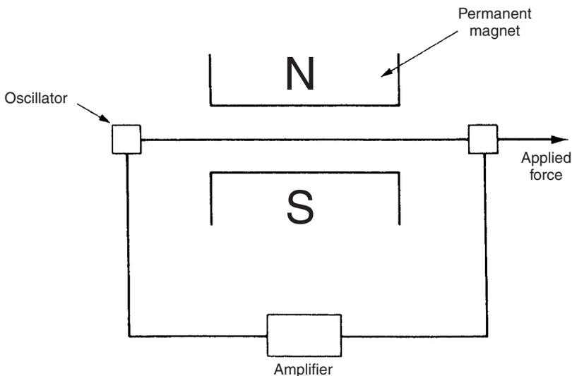
Fig. 18.9 Vibrating-wire sensor.
