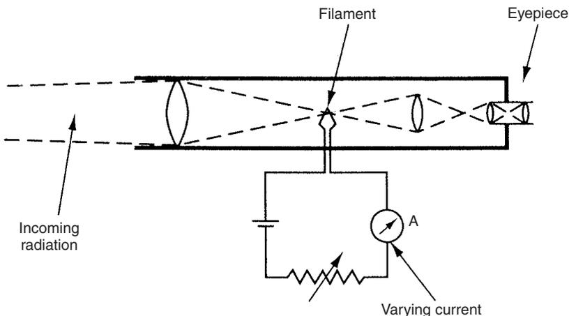
Fig. 14.11 Optical pyrometer.
