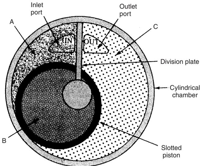
**Fig. 16.8** Rotary piston form of positive displacement flowmeter.
