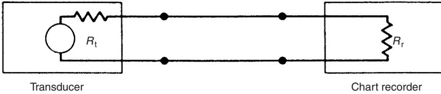
**Fig. 11.6** Connection of transducer to chart recorder.
