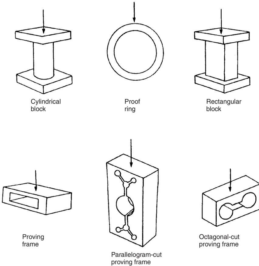
**Fig. 18.1** Elastic elements used in load cells.
