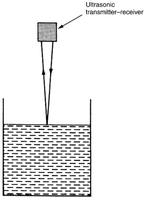
Fig. 17.4 Ultrasonic level gauge.
