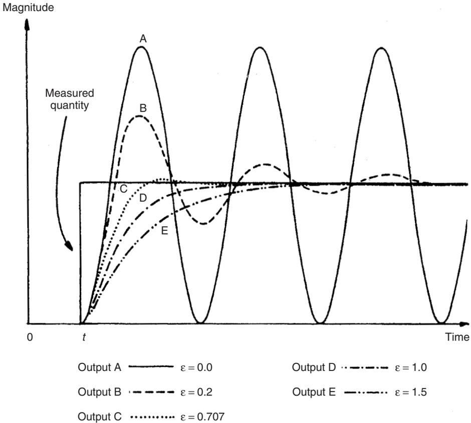
Fig. 2.12 Response characteristics of second order instruments.
