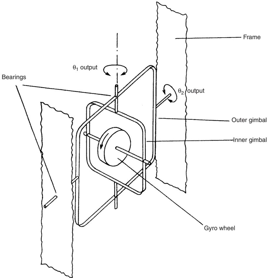
**Fig. 20.13** Free gyroscope.
