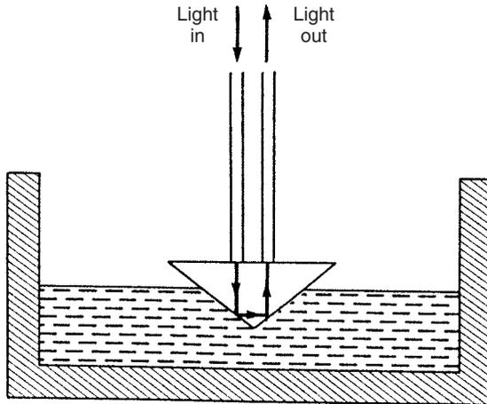
Fig. 17.12 Prism level sensor.
