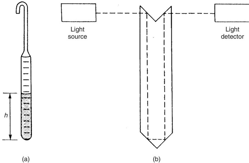
**Fig. 17.1** Dipsticks: (a) simple dipstick; (b) optical dipstick.
