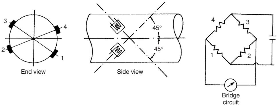
Fig. 18.12 Position of torque-measuring strain gauges on shaft.
