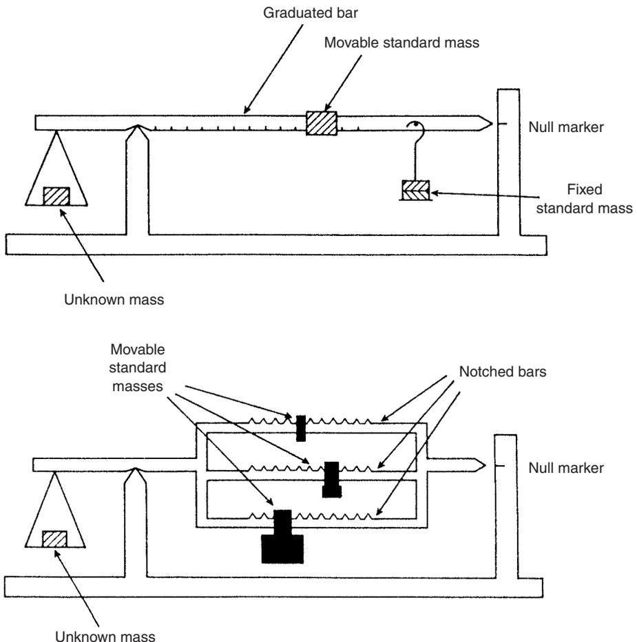
**Fig. 18.6** Two alternative forms of weigh beam.
