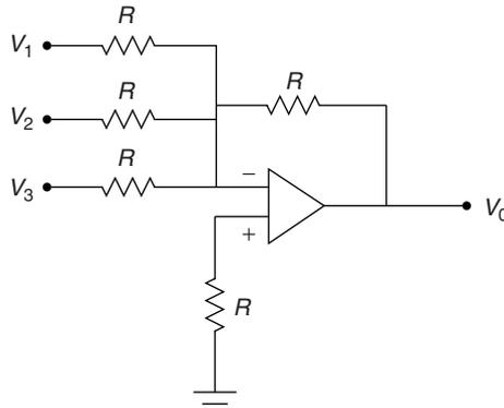
Fig. 5.20 Operational amplifier connected for signal addition.
