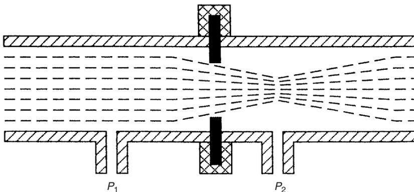
Fig. 16.4 Profile of flow across orifice plate.
