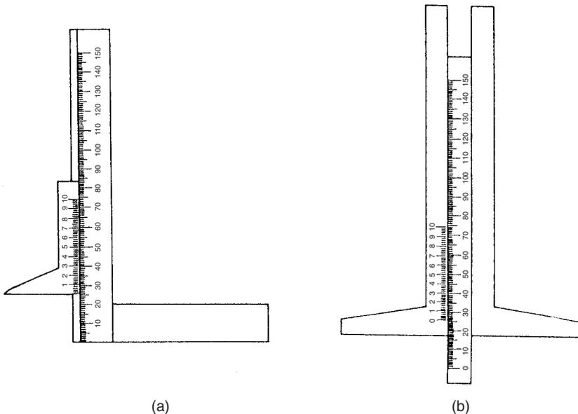
Fig. 21.7 (a) Height gauge; (b) depth gauge.
