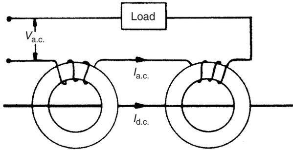
Fig. 7.15 Current transformer.
