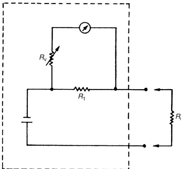
Fig. 7.11 Ohmmeter.
