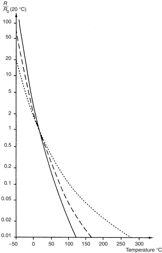
**Fig. 14.9** Typical resistance–temperature characteristics of thermistor materials.
