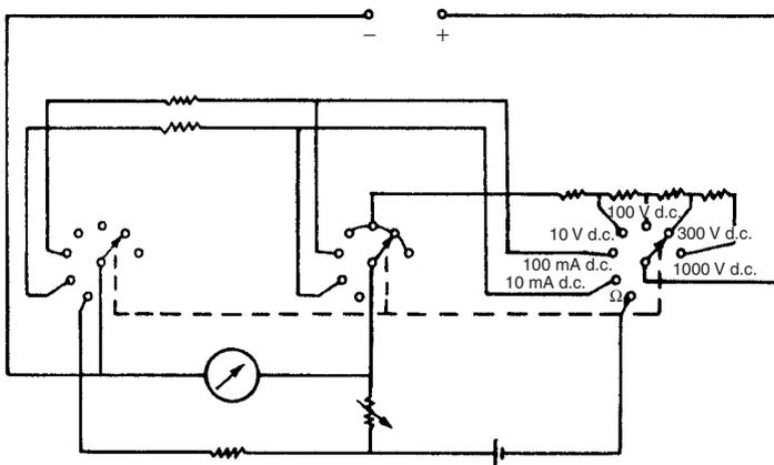
Fig. 6.6 Analogue multimeter.
