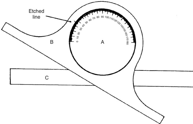
**Fig. 21.9** Angle protractor.
