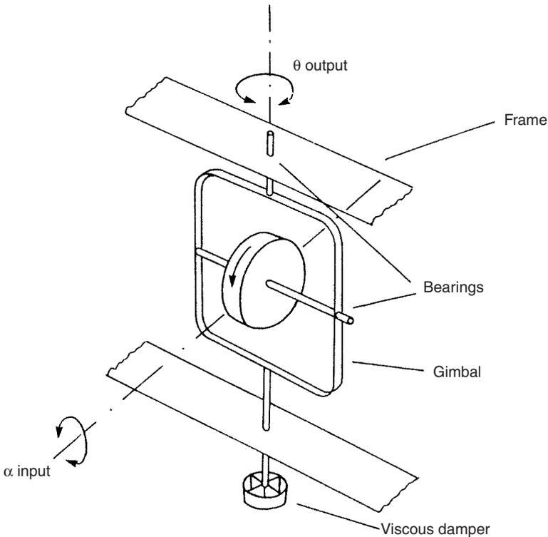
**Fig. 20.14** Rate-integrating gyroscope.
