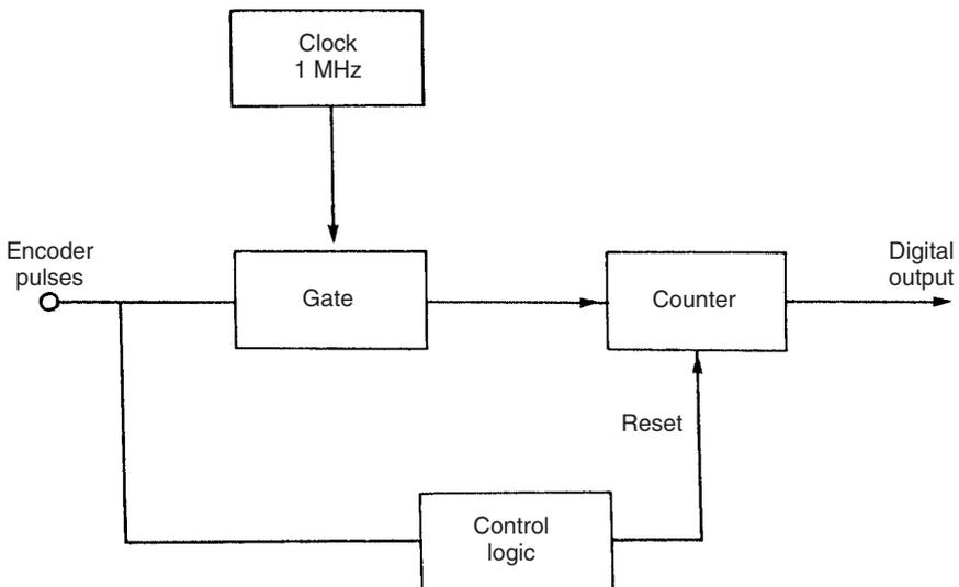
Fig. 20.16 Scheme to measure instantaneous angular velocities.
