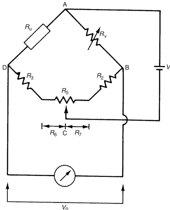
Fig. 7.6 Apex balancing.
