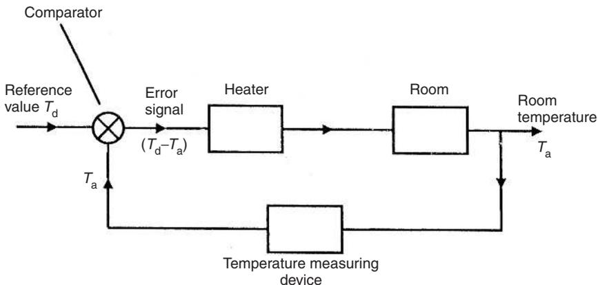
**Fig. 1.1** Elements of a simple closed-loop control system.
