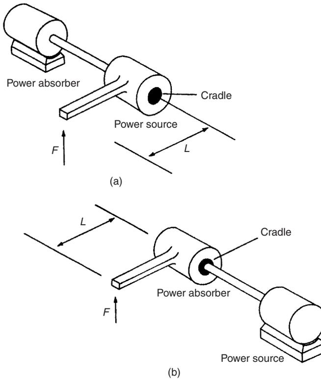
Fig. 18.10 Measuring reaction forces in cradled shaft bearings.
