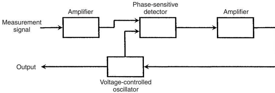
Fig. 7.17 Phase-locked loop.
