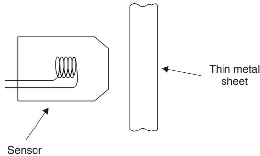
**Fig. 13.3** Eddy current sensor.
