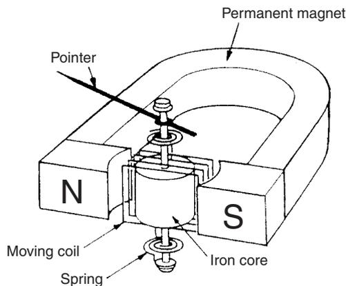
Fig. 6.2 Moving-coil meter.
