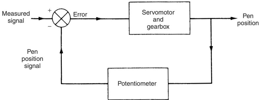
Fig. 11.8 Servo system of potentiometric chart recorder.
