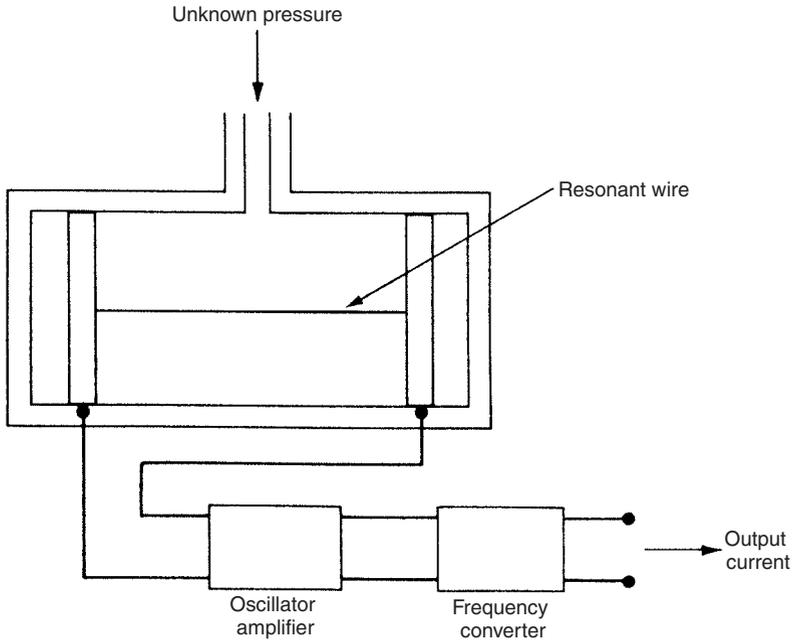
**Fig. 15.7** Resonant-wire device.
