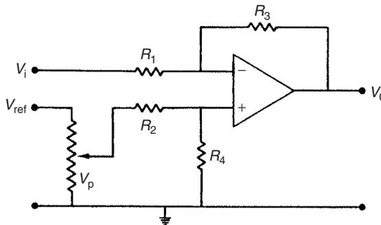
Fig. 5.14 Bias removal circuit.
