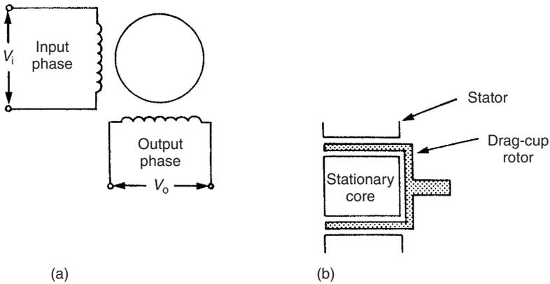
Fig. 20.20 A.c. tachometer.
