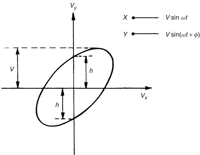
**Fig. 7.21** Phase measurement using  $X$ - $Y$  plotter.
