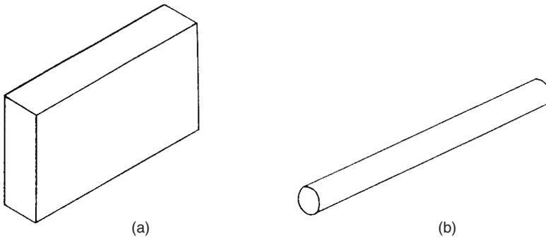
**Fig. 21.6** (a) Gauge block; (b) length bar.
