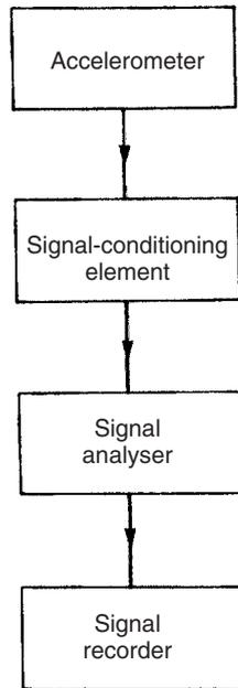
**Fig. 19.16** Vibration measurement system.
