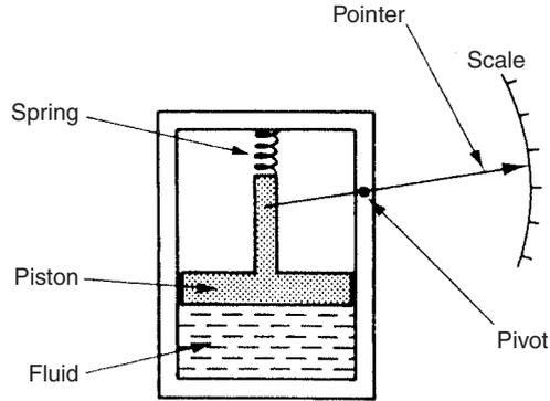
**Fig. 2.1** Passive pressure gauge.
