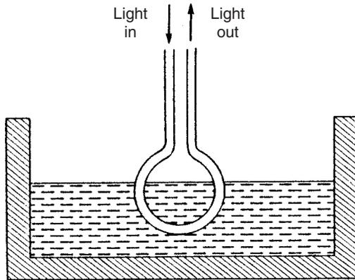
**Fig. 17.11** Loop level sensor.
