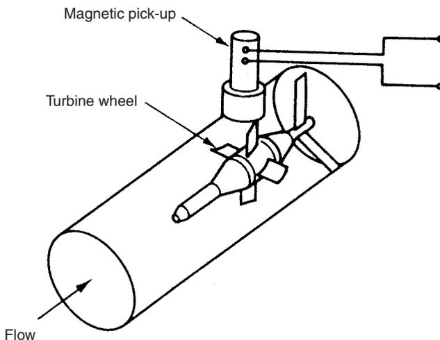
**Fig. 16.9** Turbine flowmeter.
