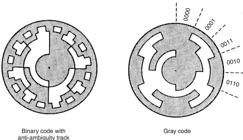
**Fig. 20.7** Modified window arrangements for the rotating disc.
