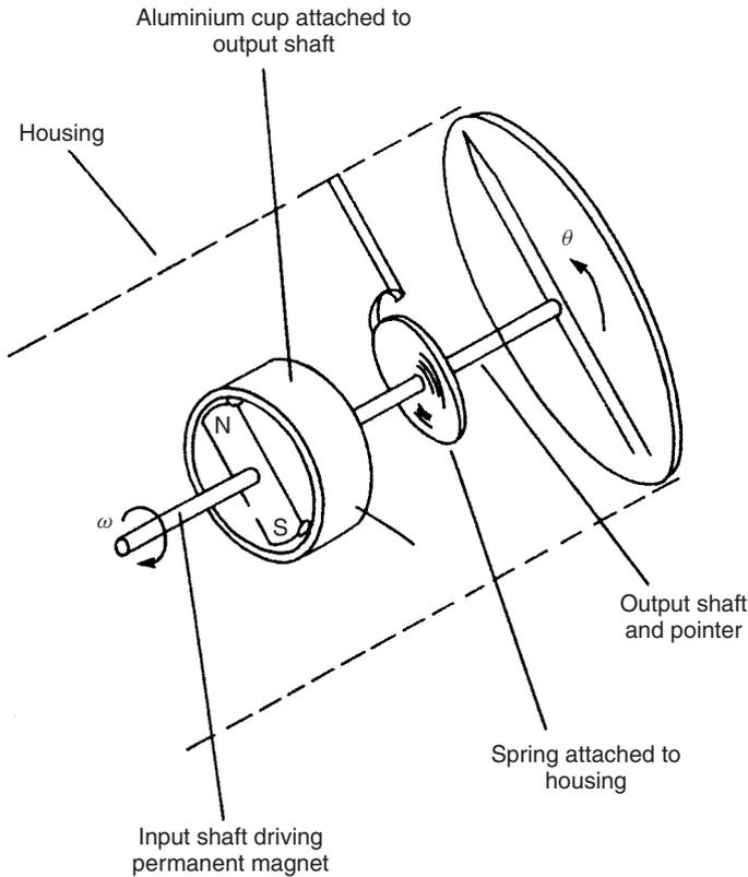
**Fig. 20.21** Drag-cup tachometer.
