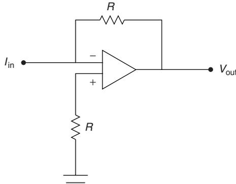
**Fig. 8.2** Current-to-voltage converter.
