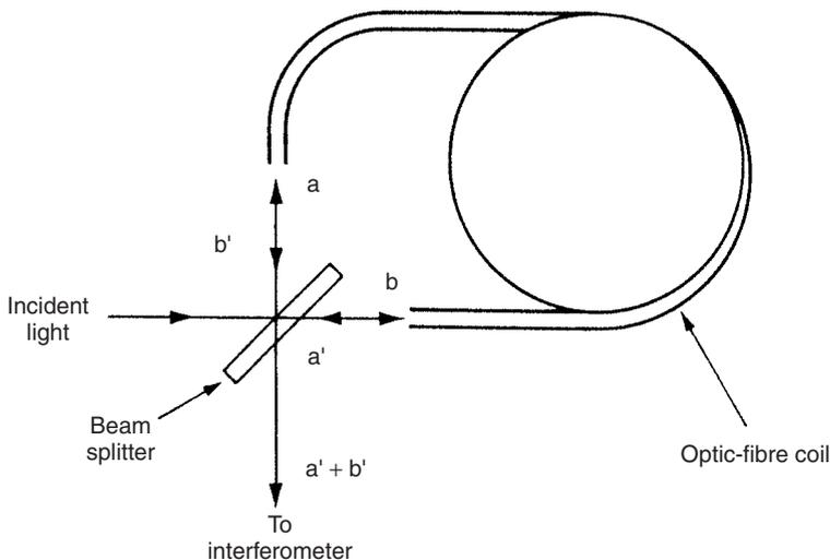
Fig. 20.24 Fibre-optic gyroscope.
