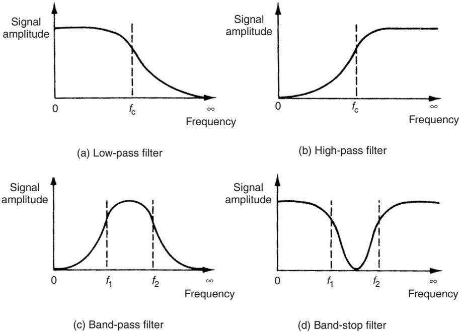
Fig. 5.5 Outputs from practical constant- $k$  filters.
