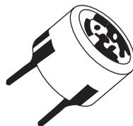
Fig. 13.10 Ultrasonic sensor.
