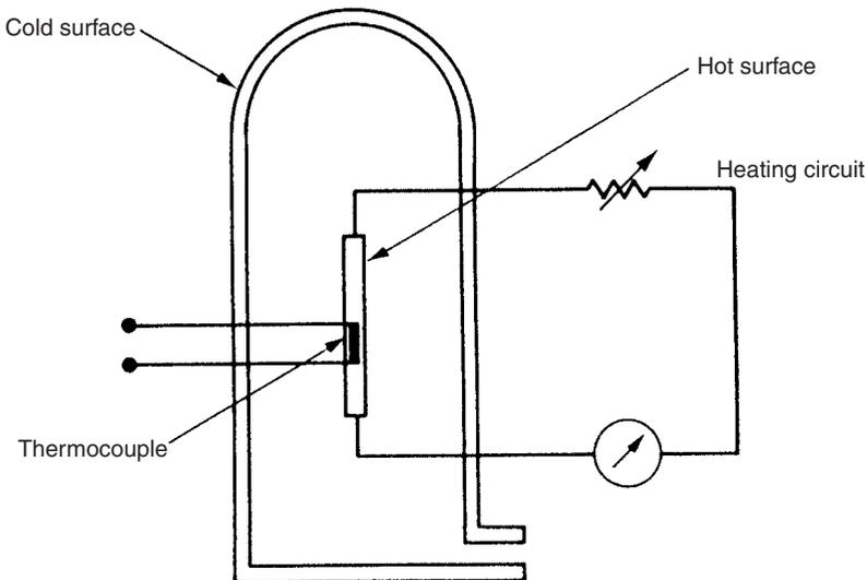
**Fig. 15.8** Thermocouple gauge.
