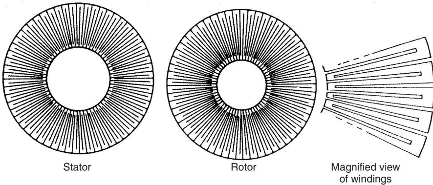
Fig. 20.12 Rotary inductosyn.
