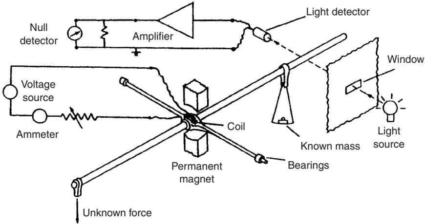
Fig. 18.8 Electromagnetic balance.
