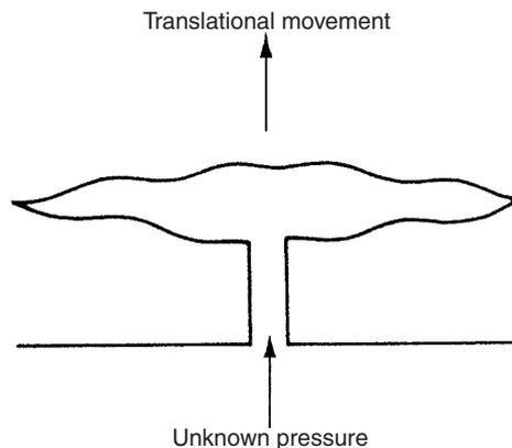
**Fig. 15.1** Schematic representation of diaphragm pressure sensor.
