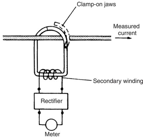
Fig. 6.5 Clamp-on meter.
