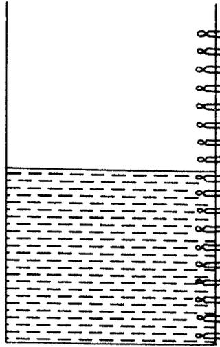
Fig. 17.9 Hot-wire-element level sensor.
