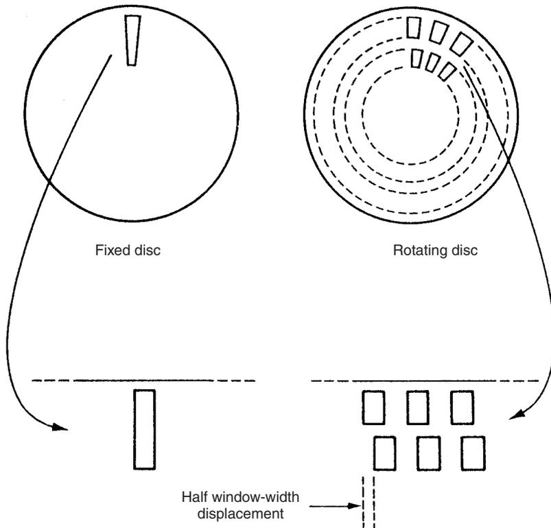
**Fig. 20.4** Window arrangement in incremental shaft encoder.
