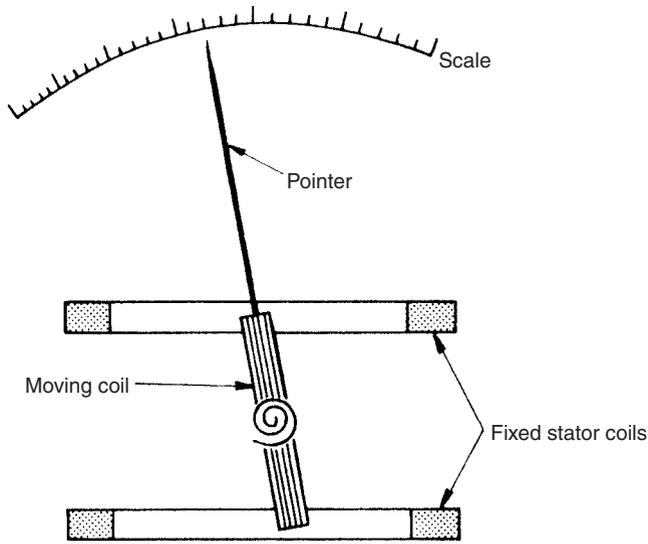
**Fig. 6.4** Electrodynamic meter.
