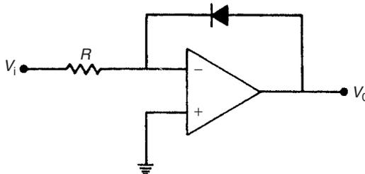
**Fig. 5.13** Operational amplifier connected for signal linearization.
