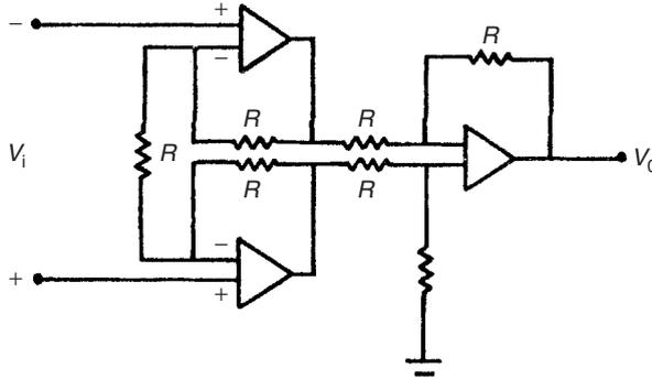
**Fig. 5.10** Instrumentation amplifier.
