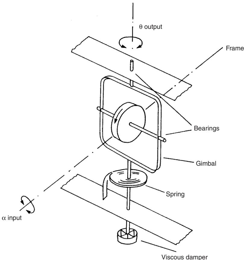
Fig. 20.23 Rate gyroscope.
