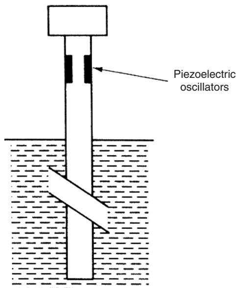
Fig. 17.8 Vibrating level sensor.
