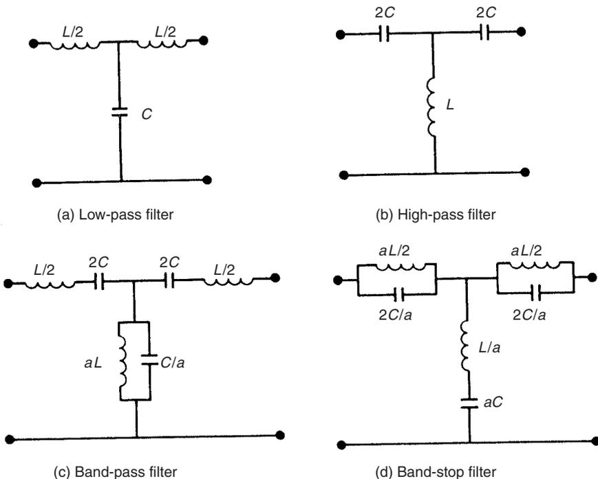
**Fig. 5.7** Circuit components for passive filter T-sections.
