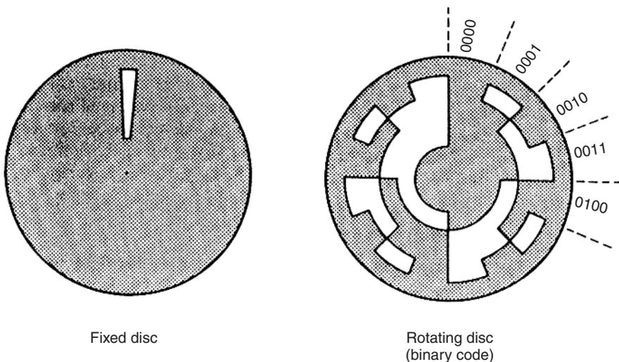
**Fig. 20.6** Window arrangement for coded disc shaft encoder.
