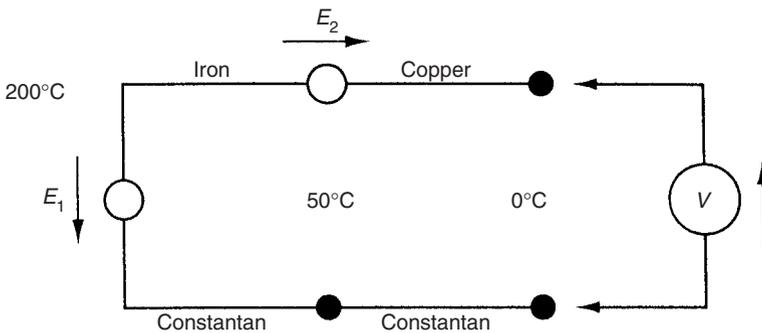
Fig. 14.6 Diagram for solution of example 14.5.
