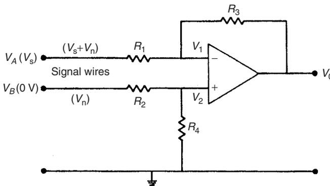
Fig. 5.12 Operational amplifier connected in differential amplification mode.
