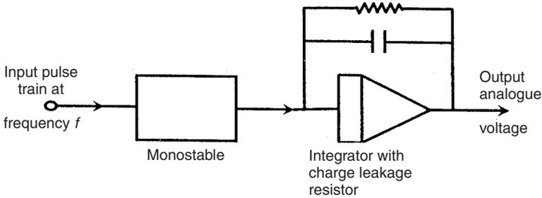
Fig. 8.4 Frequency-to-voltage converter.
