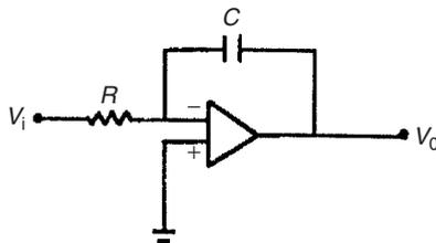
Fig. 5.15 Operational amplifier connected for signal integration.
