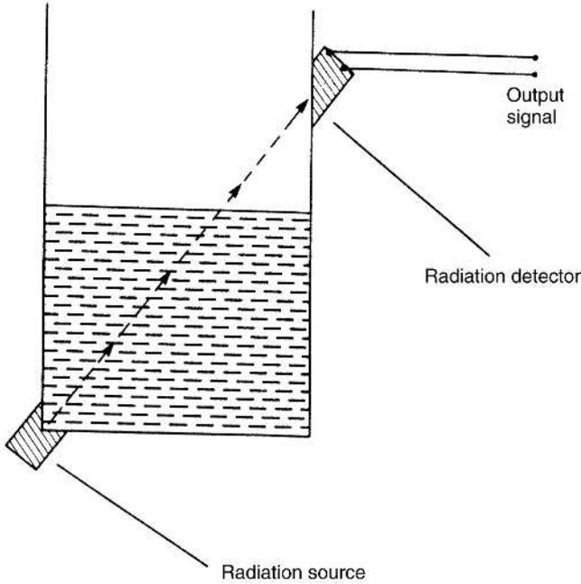
**Fig. 17.7** Using a radiation source to measure level.
