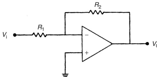
Fig. 5.9 Operational amplifier connected for signal amplification.
