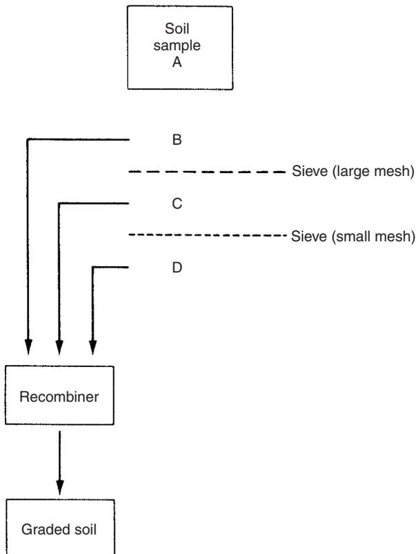
**Fig. 5.3** Soil sieving analogy of signal filtering.
