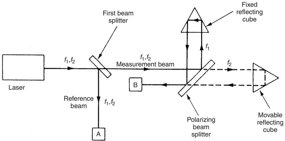
**Fig. 19.9** Laser interferometer.
