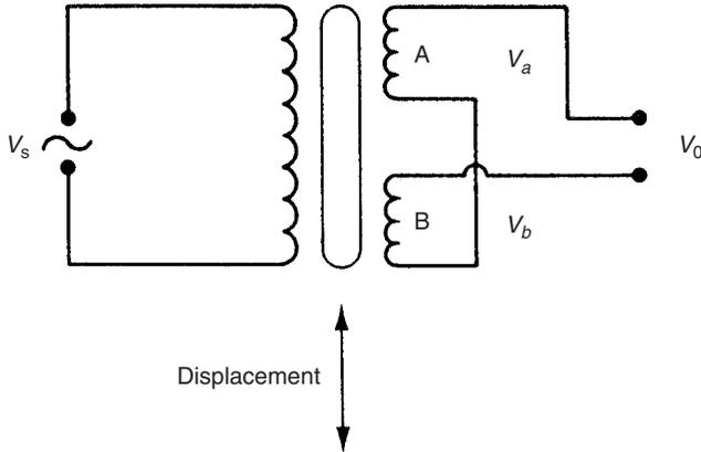
**Fig. 19.2** The linear variable differential transformer (LVDT).
