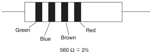
**Fig. 7.12** Four-band resistance-value marking system with example.
