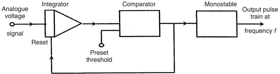
Fig. 8.3 Voltage-to-frequency converter.
