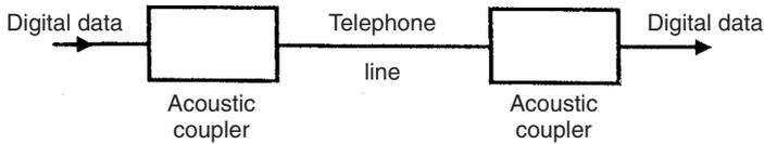
**Fig. 8.10** Telephone transmission.
