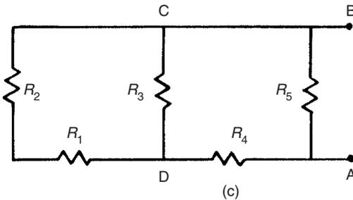
**Fig. 3.1** Analysis of circuit loading: (a) a circuit in which the voltage across  $R_5$  is to be measured; (b) equivalent circuit by Thévenin's theorem; (c) the circuit used to find the equivalent single resistance  $R_{AB}$ .
