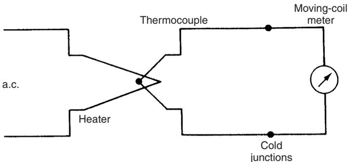
**Fig. 6.8** Thermocouple meter.
