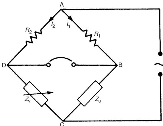
**Fig. 7.7** Null-type impedance bridge.
