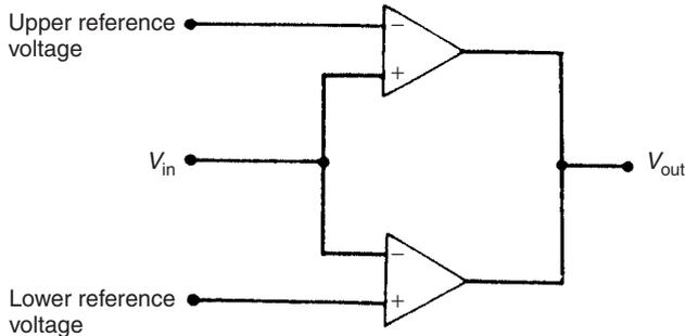
**Fig. 5.18** Comparison of input signal against reference value.
