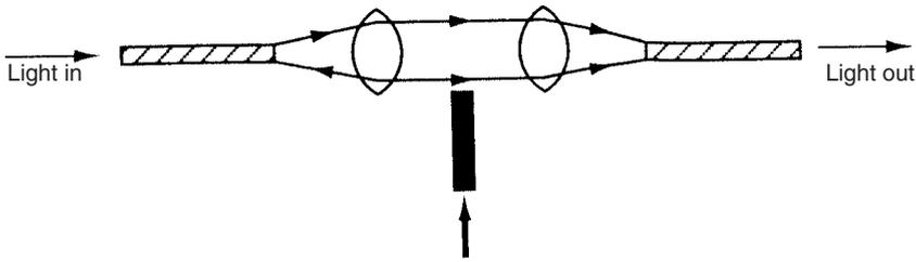
**Fig. 13.9** Variable-shutter sensor.
