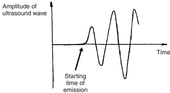
**Fig. 13.12** Ramp-up of ultrasonic wave after emission.
