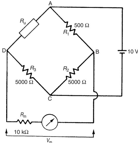
Fig. 7.5 Bridge circuit.
