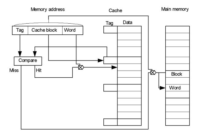
The direct mapping technique is simple and inexpensive to implement. Disadvantage: a fixed cache location for any given block.
