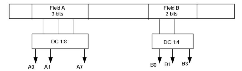
Control lines are coded into specific fields within a microinstruction.
