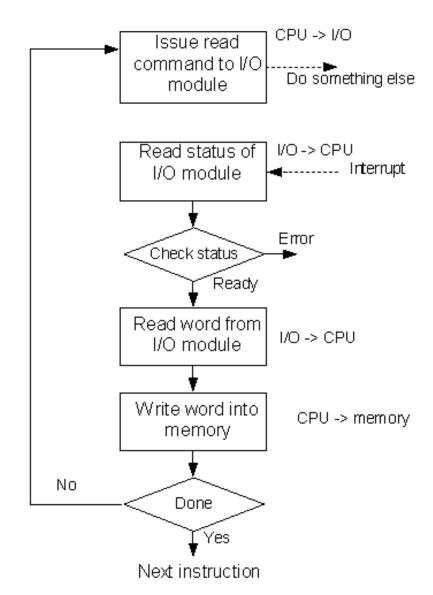
Programmed I/O and interrupt-driven I/O suffer from two drawbacks:
