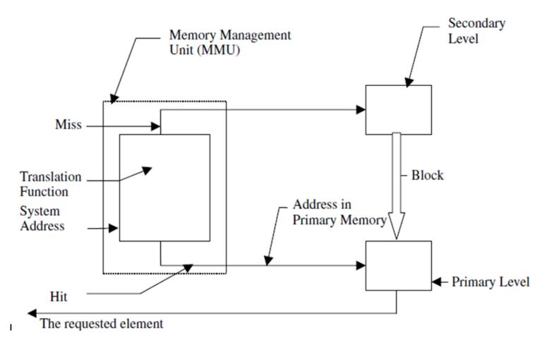
The main memory consists of up to 2<sup>n</sup> addressable words, with each word having a unique n-bit address.
