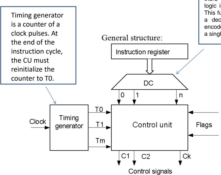
To simplify the CU logic, there should be a unique logic input for each opcode. This function is performed by a decoder which takes an encoded input and produces a single output.
