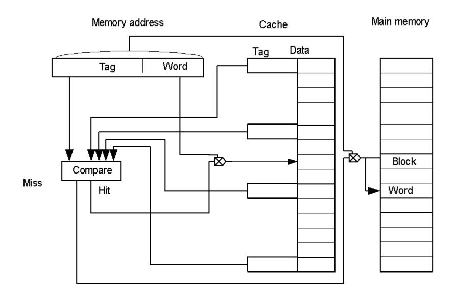
The main **advantage** of the associativemapping technique is the **efficient use of the cache.**
