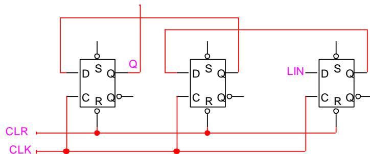
A serial-in, parallel-out shift register has outputs for all of its stored bits making them available to other circuits. Such a shift register can be used to perform serial-to-parallel conversion.
