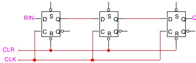
The RIN specifies a new bit to be shifted into one end at each clock tick. This bit appears at the serial output after n clock ticks. Thus an n-bit serial-in, serial-out shift register can be used to delay a signal by n clock ticks
