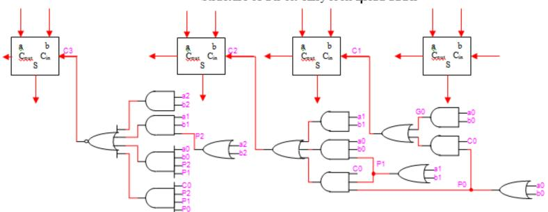
$$C_3 = G_2 + P_2 G_1 + P_2 P_1 G_0 + P_2 P_1 C_0 \qquad C_2 = G_1 + P_1 G_0 + P_1 P_0 C_0 \qquad C_i = G_0 + P_0 C_0$$
