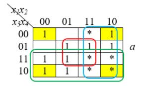
$$F_a = x_1 + x_3 + \overline{x}_2 \overline{x}_4 + x_2 x_4$$
