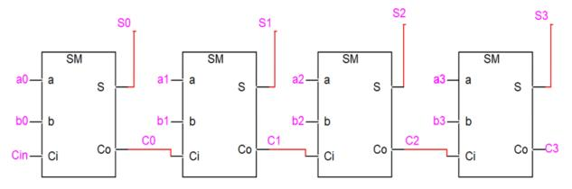
The carry input to the LSB  $C_0$  is normally set to 0 and the carry output of each full adder is connected to the carry input of the next most significant full adder.
