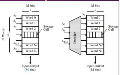
N words => N select signals Too many select signals Decoder reduces # of select signals  $K = log_2N$
