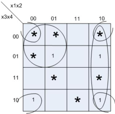
$$\mathbf{F} = \overline{\mathbf{x}}_1 \overline{\mathbf{x}}_3 + \mathbf{x}_1 \overline{\mathbf{x}}_2 + \overline{\mathbf{x}}_2 \overline{\mathbf{x}}_4$$
