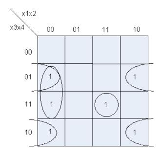
$$F = \overline{x}_1 \overline{x}_2 x_4 + \overline{x}_2 \overline{x}_3 x_4 + \overline{x}_2 x_3 \overline{x}_4 + x_1 x_2 x_3 x_4$$
