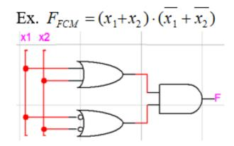
$$F_{FCM} = \overline{(\overline{x_1} + \overline{x_2}) \cdot (\overline{x_1} + \overline{x_2})} = \overline{(\overline{x_1} + \overline{x_2})} + \overline{(\overline{x_1} + \overline{x_2})}$$
