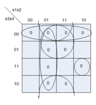
$$F = (x_1 + \overline{x}_2) \bullet (x_3 + x_4) \bullet (\overline{x}_2 + x_3) \bullet (\overline{x}_2 + x_4) \bullet (\overline{x}_1 + x_2 + \overline{x}_3 + \overline{x}_4)$$
