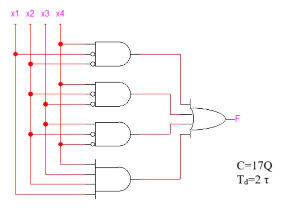
Cost (C)- the number of all inputs in logic gates. It is measured in Quines (Q). Delay time  $(T_d)$  – The number of levels in the circuit or the maximal number of logic gates that cross the signal from input to output. It is measured in  $\tau$ .
