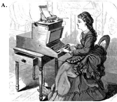
FIGURE 7.4. The 1872 Sholes Typewriter. Remington, the manufacturer of the first successful typewriter, also made sewing machines. Figure A shows the influence of the sewing machine upon the design with the use of a foot pedal for what eventually became the “return” key. A heavy weight hung from the frame advanced the carriage after each letter was struck, or when the large, rectangular plate under the typist’s left hand was depressed (this is the “space bar”). Pressing the foot pedal raised the weight. Figure B shows a blowup of the keyboard. Note that the second row shows a period (.) instead of R. From Scientific American’s “The Type Writer” (Anonymous, 1872).
